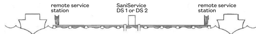
This diagram shows the layout with multiple hose stations connected to a single pump. This allows two or more users of a pump and may be set up to allow for remote operation. Careful design of this configuration is needed for optimal performance.
