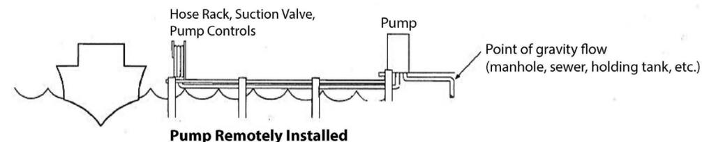
This diagram shows the pump as two separate entities. The hose rack is at the point of service while the pump is set apart, either at the end of the dock or it can be located landside.
