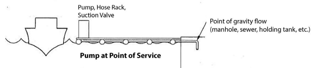
This diagram shows the pump system (hose rack and pump) as one unit, at the point of service.
